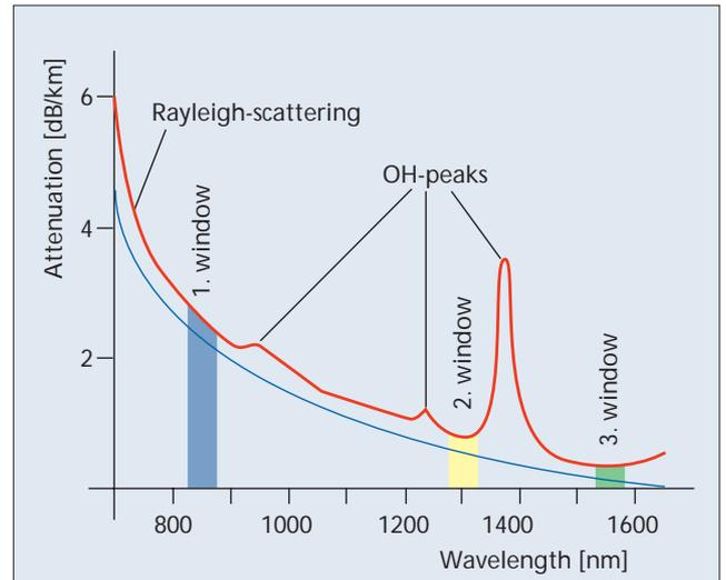
Attenuation characteristics of optical fibres at different wavelengths
