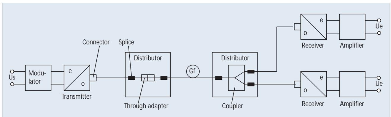
Principle of an optical transmission route
