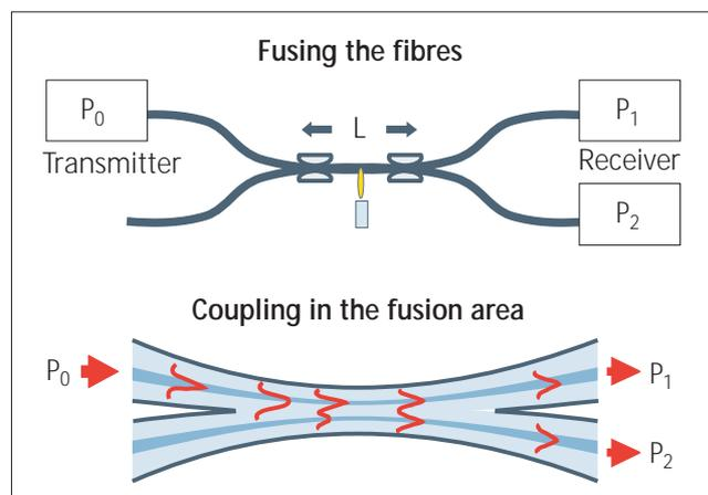
Production and operating principles: fusing the fibres (top) and coupling in the fusion area (bottom).
