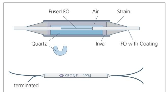
Schematic structure of a fused coupler
