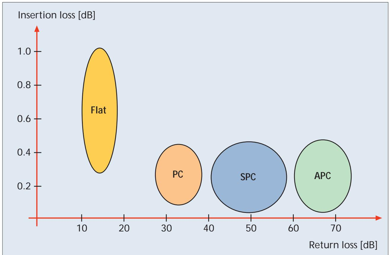
Insertion and return loss as a function of the connector face area
