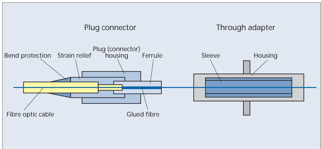
FO plug connection based on the pin-and-sleeve principle
