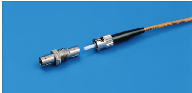
The straight tail (ST) connector was developed by AT&T. It is the type most frequently used in LANs, and is internationally standardised as a multi-mode connector. In the USA, however, the Bell Operating Companies also use it as an SM connector.
