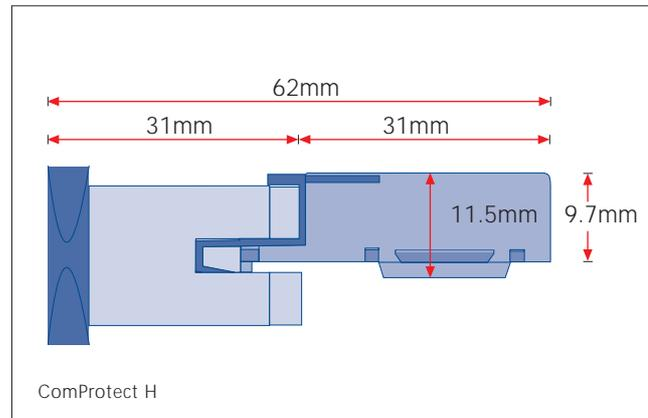
Dimensions of a ComProtect 1-pair protective plug (type A, B, C, D and H) installed in the LSA-PLUS distribution module
